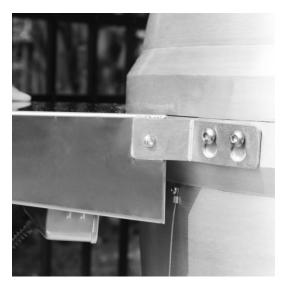
2. Once the shelf brackets are properly positioned over the fasteners, tighten the fasteners with a #5 mm allen wrench.
