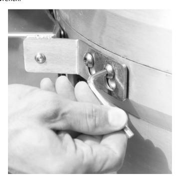
3. Underneath the shelf, you will find a shelf leveling / stabilizing screw. This screw holds tension against the grill body leveling the shelf and holding it securely in this position. Tighten this screw using a #6 mm allen wrench. When complete, the shelf should be level. See below:
